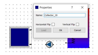
When a three-way valve is placed, the darker connector indicates the port through which there is always flow, when there is flow at all. In our case this needs to be towards the warm water tap, since the three-way valve placed is supposed to be the mixing valve for the warm water demand. To access the valve settings the component is simply double-clicked. In the opened dialogue "vertical flip" is ticked for the correct orientation of the valve and "tempering valve" to make it one.
