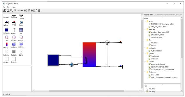
Components are simply added to a diagram by dragging the respective item from the library on the left into the central widget. It is recommded to toggle the snap grid for placing components to ease the alignment of them:
