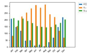
monthlyBalance Custom monthly balance. The sign of the values can be inverted by adding a - in front of the variable name. If positive and negative values don't add up to zero, the imbalance is shown as black bars. The name of the pdf to be created needs to be specified through pdf name. When adding the optional style:relative the bars will be shown as values relative to the positive sum of the monthly energy values:
