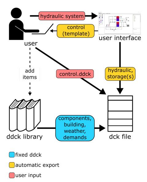
ddck-files that are specific to each system can be directly exported from the graphical user interface. These are the thermal storage tank(s) and the hydraulic information of the system. Furthermore, a template for the control.ddck can be exported from the graphical user interface, of which the details need to be filled by the user directly. Finally, a user can also create any kind of ddck-file specific to their needs from scratch.
