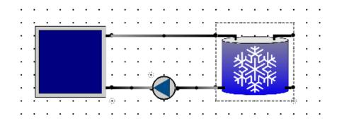
Connections can be created by moving the cursor over a port, pressing the mouse, and dragging the cursor to the port that is supposed to be connected, and release the mouse there. Each pipe has a technical flow direction along which the mass flow rate is considered to be positive (and negative if it goes in the opposite direction). The technical flow direction is indicated by a gradient going from a bright to a darker grey along the positive direction.
